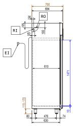
Electrical inlet (power) Refriaerant Inlet Refrigerant Outlet
